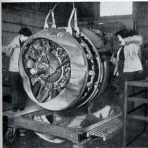
Fig. 239—In the Power Plant Bay, starting to dismantle the ancillary equipment from a Wildcat Cyclone 9 cyl. engine after a barrier crash in a carrier.
