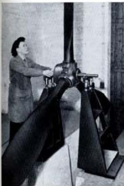
Fig. 231—Testing the static balance of a 13ft. 6in diameter Hamilton Hydromatic propeller.
