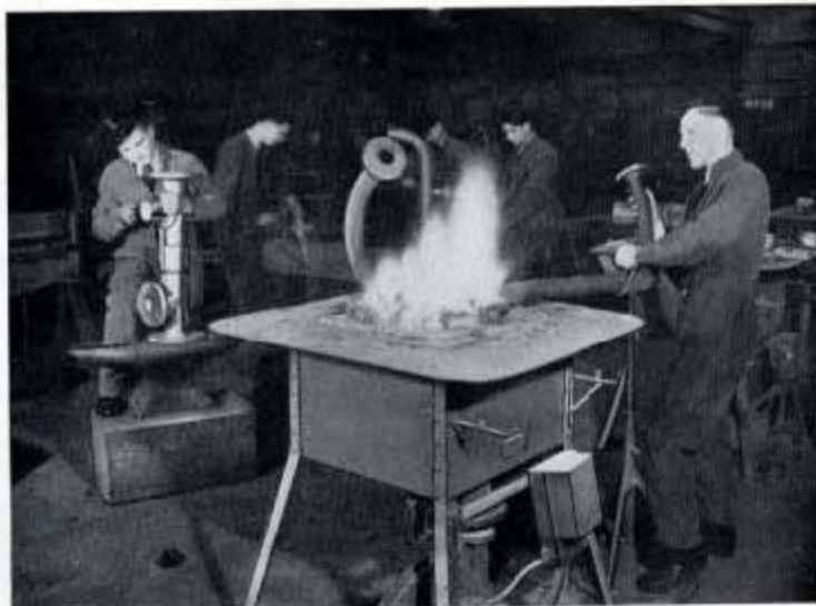
Fig. 68—Coppersmiths at work. On the front forge is the C Class test job (see F, Fig. 66) whilst the apprentice at the anvil is finishing one of his Admiralty passing out test jobs (see C, Fig. 79). On the rear table a B Class test job is being built up as E, Fig. 66.
