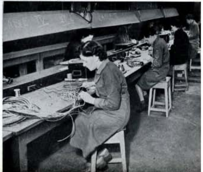
Fig. 263 (Right)—On these benches new connector sets are in process of manufacture; the woman in the foreground is using an electric soldering iron.
