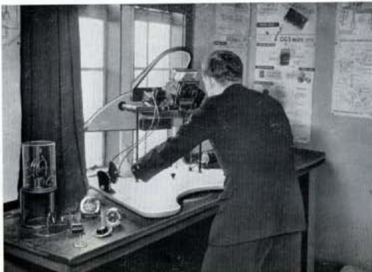
Fig. 184—Here we see instruction being given to electrical maintenance ratings on the Barracuda D.R. (distant reading) Gyro-Magnetic Compass, together with the series of repeater compasses for pilot and observer.
