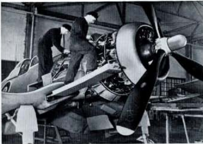
Fig. 208—Two engine fitters at work in the A.R.S. (airframe repair section) using the standard platforms provided by the manufacturers. The front one fits into the stub plane and nose cowling, the rear one is necessary owing to the steep slope of the wing roots.
