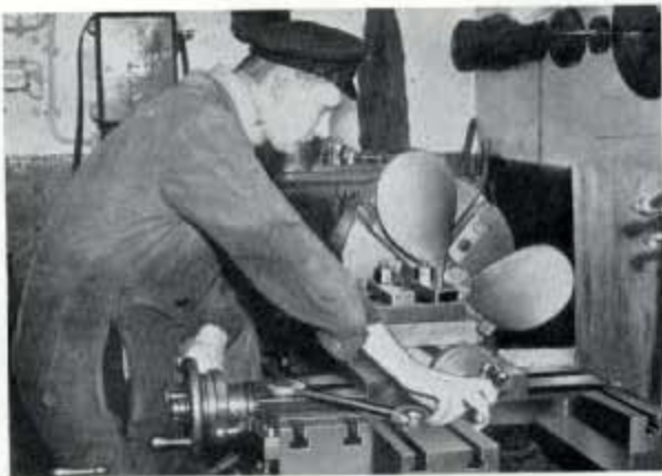
Fig. 145—Turning the propeller boss on a Lang lathe prior to the boring operation; the propeller was cast in the ship's foundry.
