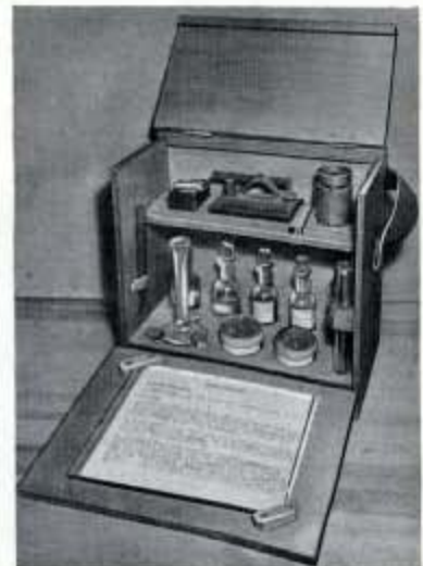
Fig. 180—This portable testing apparatus was made on the Station for the Officers Conversion Course for diagnosing metal removed from an engine filter to assist in determining the cause of failure.
