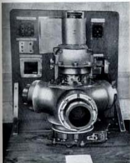
Fig. 218—This Curtiss electric propeller demonstration rig is situated in the Electrical Workshop; when a power unit has been stripped, serviced and re-assembled, it is mounted on the propeller boss in place of the sectioned model and given a complete functional test.
