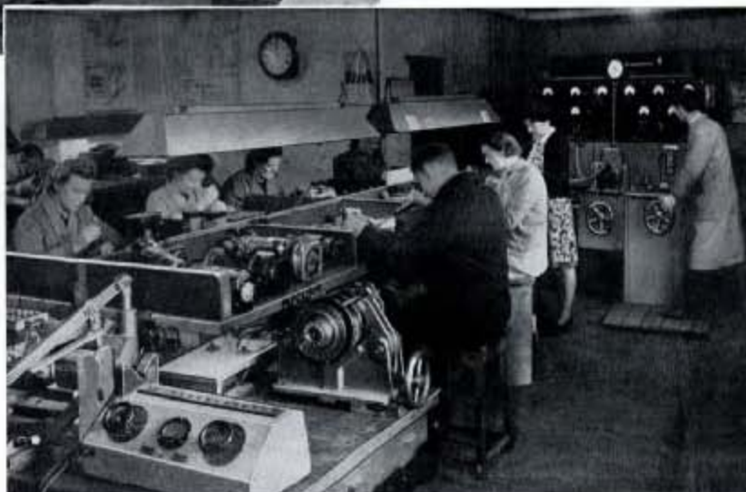
Fig. 255—The Electrical Division handles all electrical matters pertaining to aircraft. Here is part of the Repair Shop where generators, alternators, starters, regulators, etc., are overhauled, repaired and tested.
