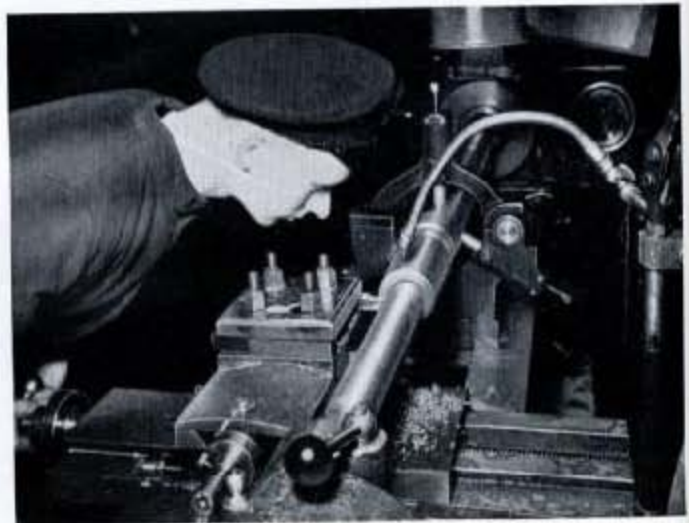
Fig. 42 (Right) — The apprentice in the early stages of turning the main circulating pump shaft.
