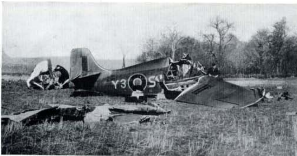
Fig. 283—A pupil Pilot Officer crashes this Wildcat shortly after taking off from the No. 1 Naval Air Fighter School at Yeovilton; after an inspection, the Aircraft Salvage Section is notified to bring in the wreck for ultimate reduction to "spares and produce."
