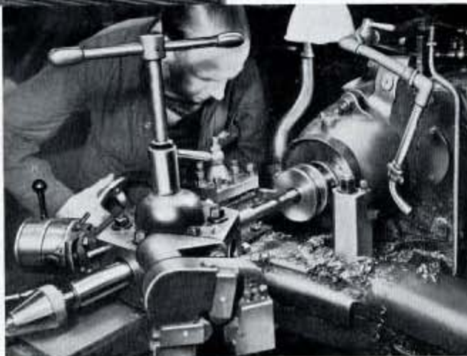
Fig. 270—A vee pulley is required for a portable hydraulic test rig, so it is machined all over on the Ward No. 2A Capstan Lathe as illustrated.
