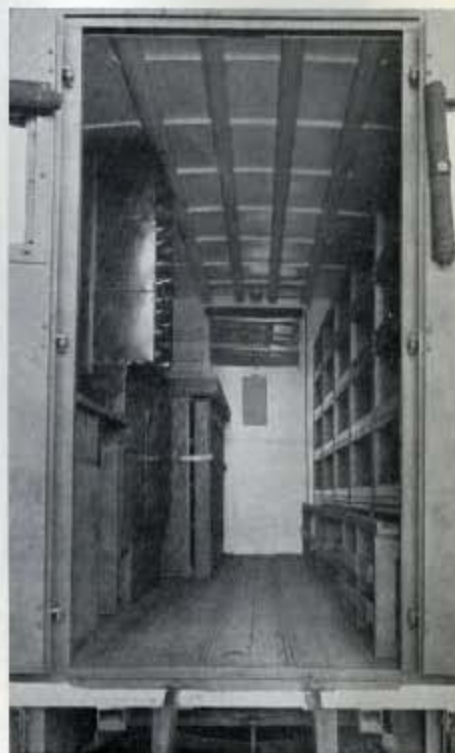
Fig. 323—An interior view of a M.S. Universal Store Lorry showing the stowage arrangements for all types of aircraft stores.
