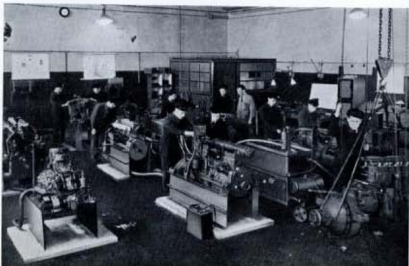
Fig. 49 (Right)—I.C.E. instruction for Fitters and Turners covers 10 weeks training (5 weeks F Class, petrol and paraffin engines, and 5 weeks G Class diesel engines). In this running shop, faults are laid on and have to be traced and rectified.
