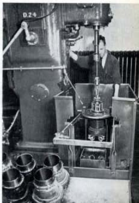
Fig. 248—Honing a worn Mercury cylinder; the bore can be taken to .010" above normal for standard pistons with new rings.
