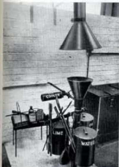
Fig. 280—A handy air blast coke fire for the heat treatment of tools.
