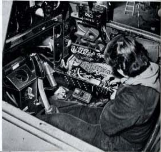
Fig. 258—An E.A.S. (electrical assembly section) mechanic tightening and checking connections on the main distribution and fuse panel in the pilot's cockpit of an Avenger.
