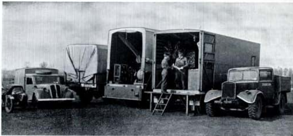
Fig. 217—Here we illustrate the equipment of a Corsair S.S.U. (squadron servicing unit). This was originally attached to the Station to supply stores during the transitional period to Corsairs and can service a Squadron of twelve aircraft for 14 days.
