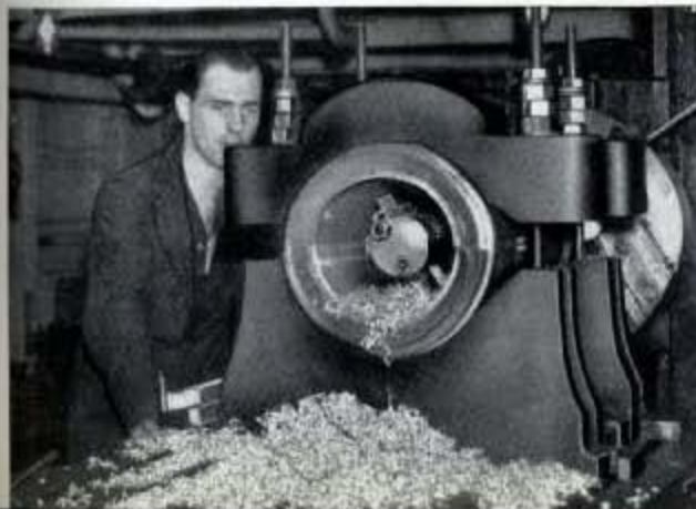
Fig. 149 (Below)—Boring the top and bottom halves of a 9" bore main engine bearing for a cruiser.
