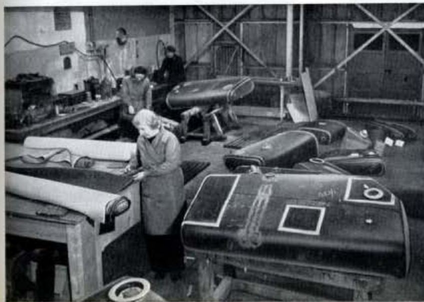
Fig. 268 (Left)—This Tank Shop is another section of the Mechanical Workshops and here can be seen self-sealing and metal petrol tanks in course of repair.
