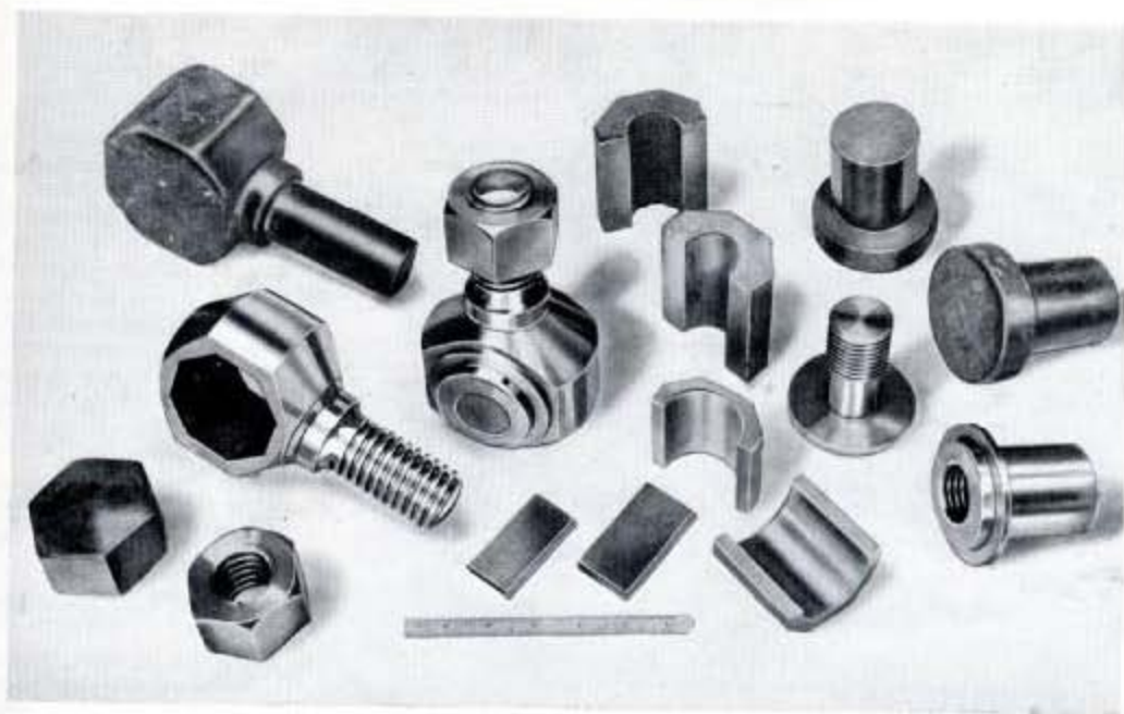
Fig. 55—The third example of Admiralty passing out test jobs for Fitters and Turners here features the gudgeon end. On all four tests, milling and slotting machines are not allowed and slotting must not be done in the lathe; chasers, taps, stocks and dies are also forbidden.
