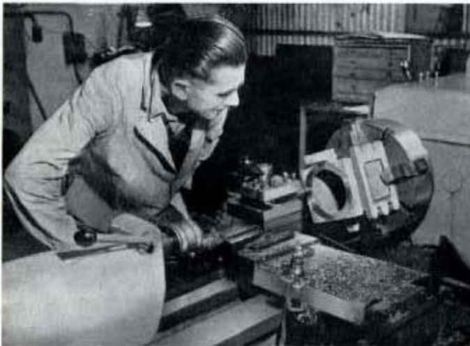
Fig. 295—A turning operation on an altimeter test chamber for use in the Instrument Shop (see Fig. 303).
