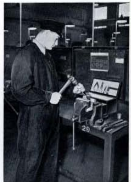
Fig. 30—R. A. Edmonds, a new entry apprentice from Birmingham, commences work at his allotted bench position on a simple chipping operation; his issued kit of tools stands open at the rear of the vice.
