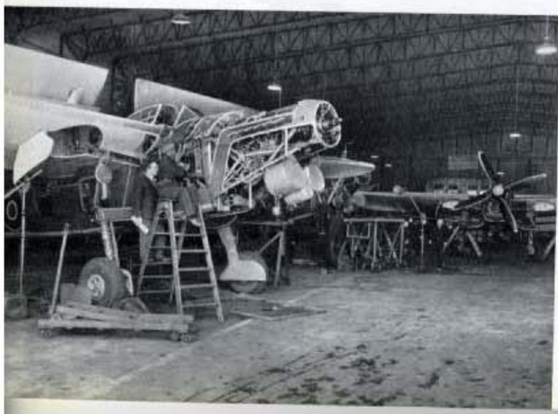
Fig. 244 (Left)—Minor and major inspections as well as airframe maintenance work being carried out in Assembly I hangar, devoted to Barracudas only.
