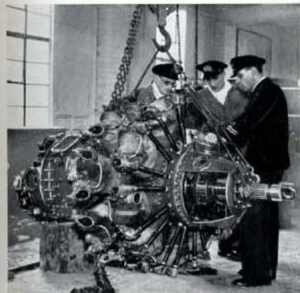
Fig. 134—A sectioned 18 cylinder Double Wasp engine of 1,675 rated horse power for a Hellcat fighter aircraft being used for instructional purpose in the Engine Repair Section.
