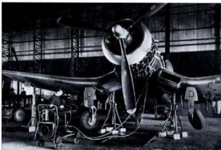
Fig. 206—This Corsair made a heavy landing on the drome so it is now undergoing an undercarriage retraction test with the use of a hydraulic test rig in No. 1. Maintenance Unit hangar.
