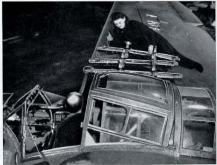
Fig. 261—E.A.S. mechanics checking and testing the bomb installation of a Barracuda for correct firing rotation; for convenience the bomb racks are placed on top of the main planes.
