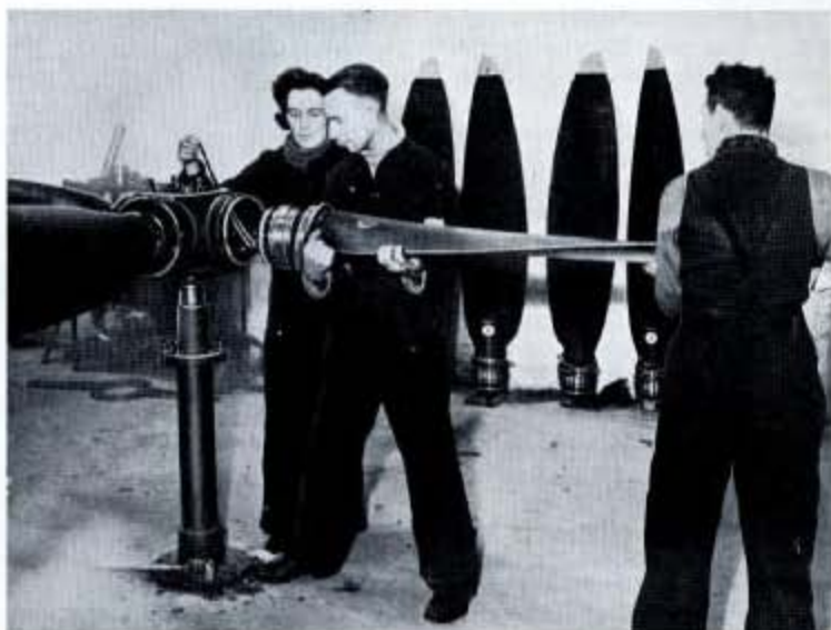
Fig. 232—Assembling a Rotal four-bladed propeller for a Barracuda, the woman assists by guiding the operating link through the hub shell by means of a cord.
