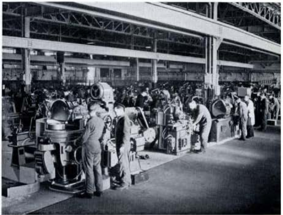
Fig. 31—A general view in the Factory Machine Shop; a Churchill Piston Ring and Surface Grinder will be seen at work in the foreground.
