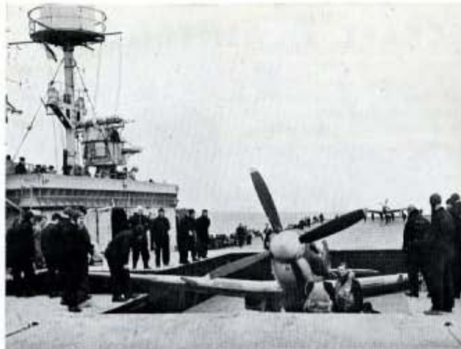
Fig. 338—Seafires being brought up from the hangar for ranging on the flight deck of an aircraft carrier.
