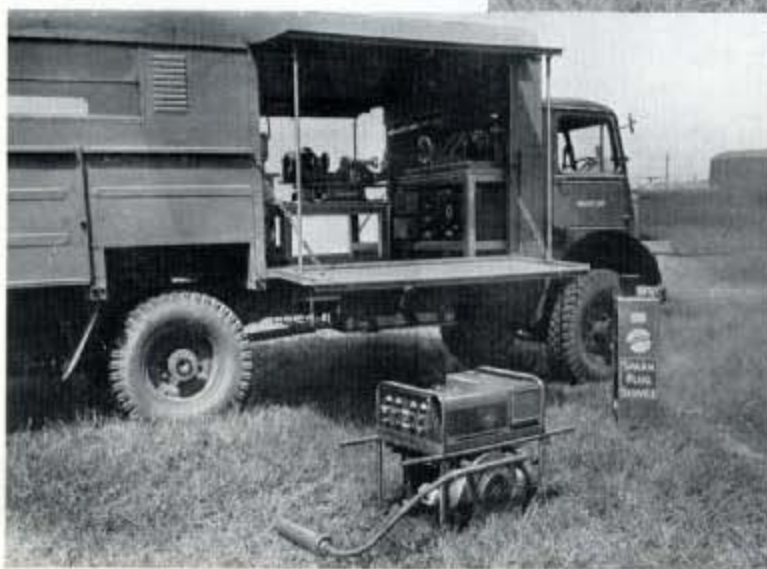
Fig. 321—This Electrical and Instrument Workshop completes the M.O.N.A.B. Mobile Maintenance Component. In the foreground will be seen a portable petrol driven generator test set and sparking plug servicing unit.
