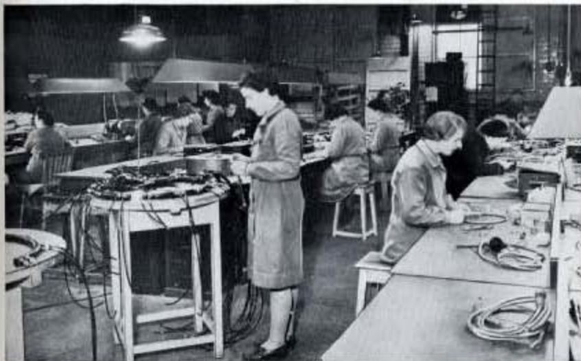
Fig. 262—A general view in the Dunfermline Ancillary Repair Shop which deals with electrical harness and sparking plugs, also the complete manufacture of new connector sets.
