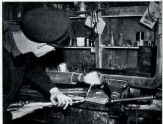
Fig. 155—A welding job for the coppersmith who gets to work with his oxy-acetylene equipment.
