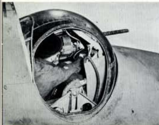
Fig. 350—Before the Board of Survey make their inspection of the aircraft on the flight deck, the guns are removed together with the wireless, safety and other equipment; here will be seen an Air Mechanic (O) from the Air Ordnance Workshops, removing the .3 Browning turret gun from an Avenger.
