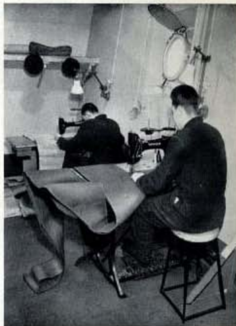
Fig. 359—These mechanics in the Fabric Workers Shop are at work on canvas lifting stroops for stowing aircraft main planes. This shop deals with all aircraft fabric repairs.
