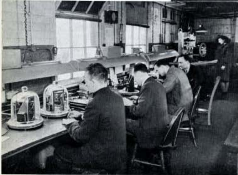
Fig. 257—A view in the Instrument Repair Shop which deals with the maintenance and test of altimeters, air speed and engine speed indicators, rates of climb indicators, oxygen equipment, etc.
