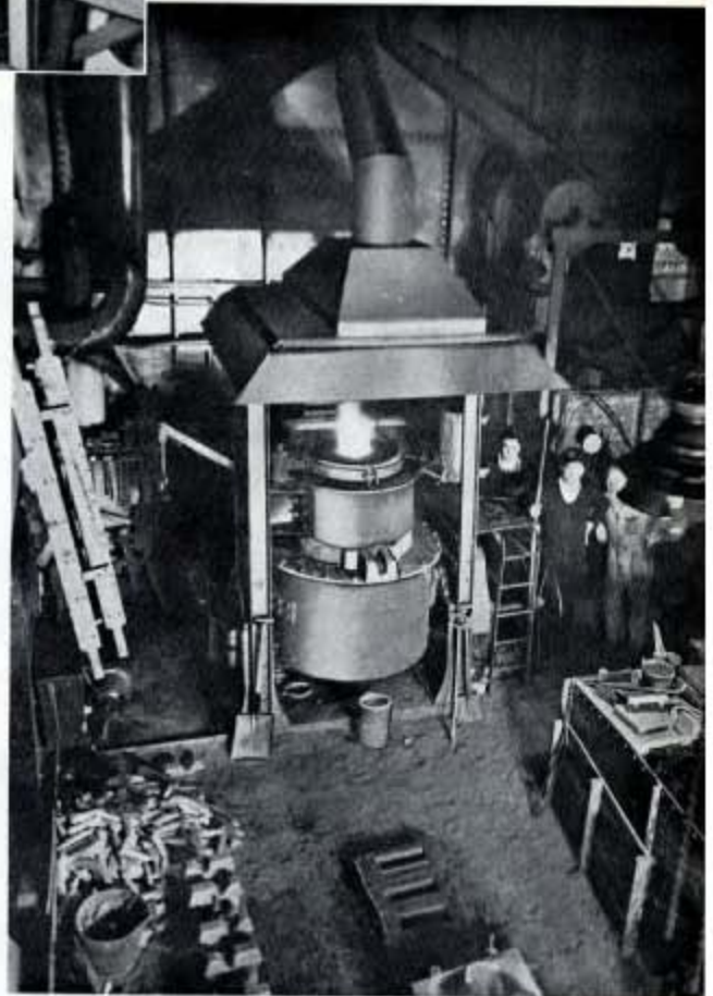
Fig. 159—This gives a good view in a typical Repair Ship Foundry; the cupola is nearly ready for pouring.
