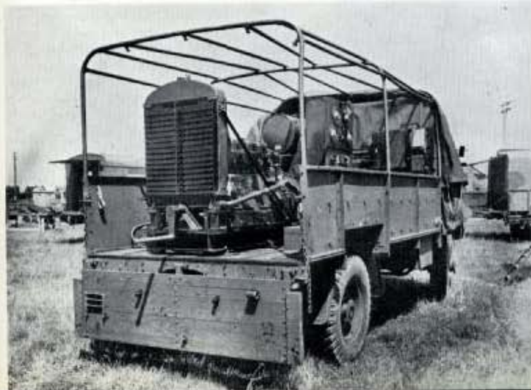
Fig. 316—This view, taken from the right hand side of the Aircraft Machine Shop, shows how the side doors let down offering extra work benches if required, as well as cooler working conditions in hot climates.
