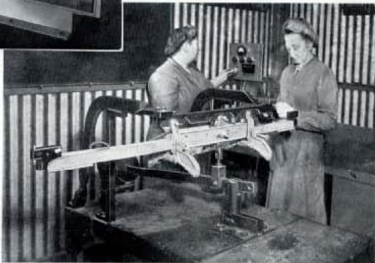
Fig. 299—A universal bomb carrier rig for testing the circuits of bomb release gear.
