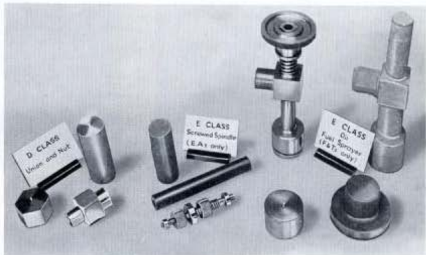
Fig. 37—Here are the next progressive test jobs covering lathe practice which follow the bench test jobs in Fig. 33; left—½" union and nut (D Class, Fitters and Turners and Electrical Artificers); centre—screwed spindle (E Class, 2 to 2½ year period, Electrical Artificers); right—oil fuel sprayer (E Class, Fitters and Turners).
