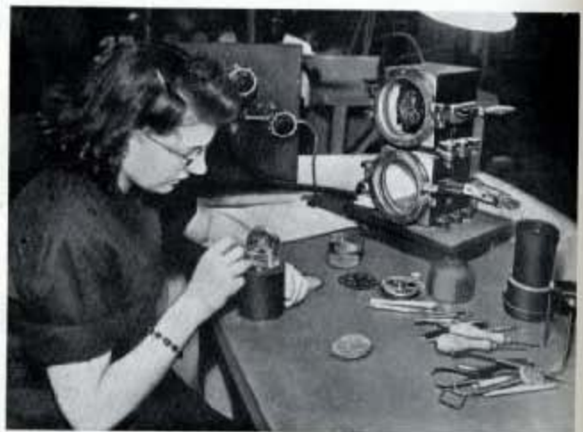
Fig. 303—Here we show in use two of the altimeter test chambers previously seen under manufacture in the Machine Shop section (Fig. 295).
