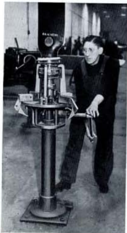
Fig. 229—A standard Rotal tool for fitting the bearing assembly to the blade the correct way up, with the smaller ball race at the top.
