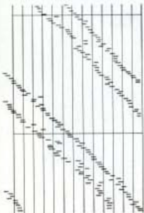
Fig. 306—This portion of tape from the Timegraph shows that the watch on test was slow at the rate of 75 seconds per day.
