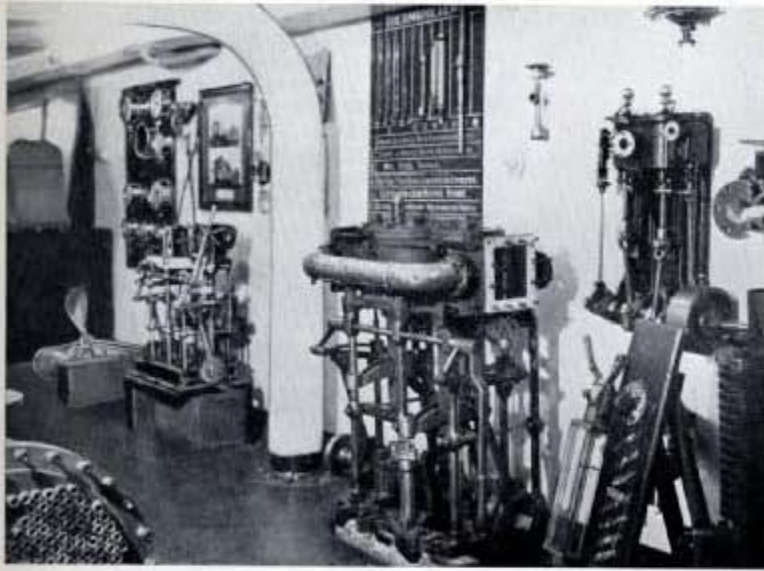
Fig. 16—Small compound reciprocating engines together with various types of thermometers, pressure and vacuum gauges in the Machinery Demonstration Room.
