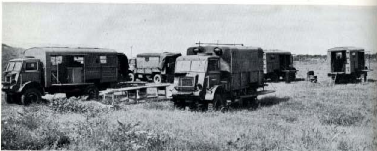
Fig. 314—A general view of a M.O.N.A.B. Mobile Maintenance Component comprising aircraft machine shop, two generator lorries, battery charging lorry, general purpose workshop and electrical and instrument workshop.
