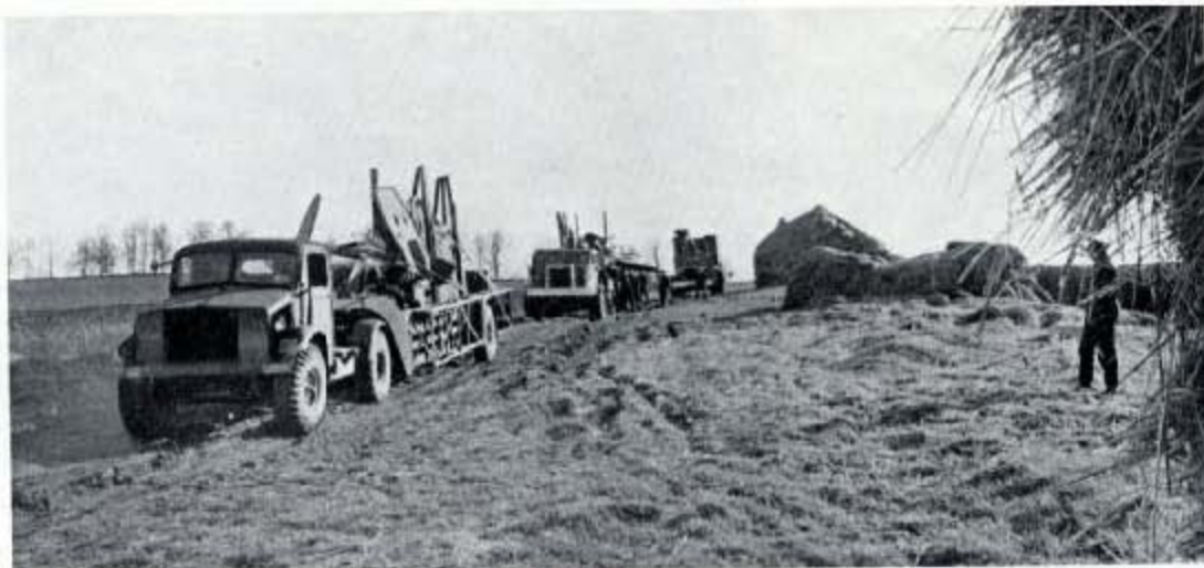
Fig. 286—The articulator with engine and main planes and the Cat truck with the fuselage, journey from the scene of the crash across the field road, the Neals crane bringing up the rear.
