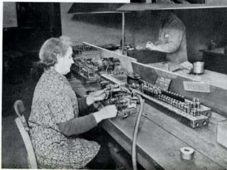
Fig. 265—Three different types of self-contained motor driven spinners running at 1,500 r.p.m. for cleaning the cases, threads and electrodes, respectively, of sparking plug components.
