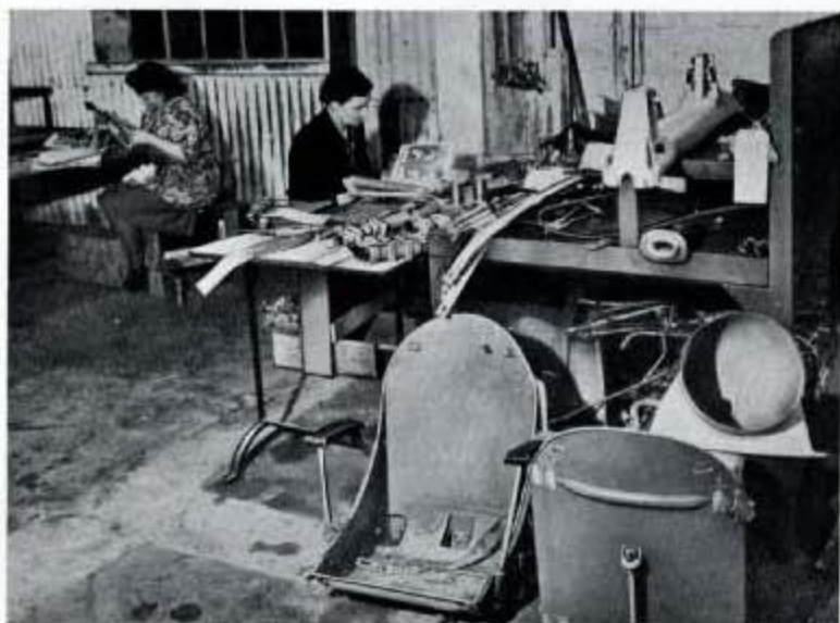
Fig. 291—Identifying serviceable Hellcat components at the Alloa Recovery Depot by means of a photographic stores catalogue in which every item on the aircraft is illustrated.
