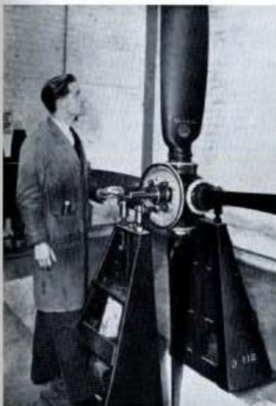
Fig. 234—An Aircraft-Repair Inspector passing the static balance of a 10ft. 5in. diameter Rotal four-bladed propeller, which must be correct to within a 3 inch ounce.
