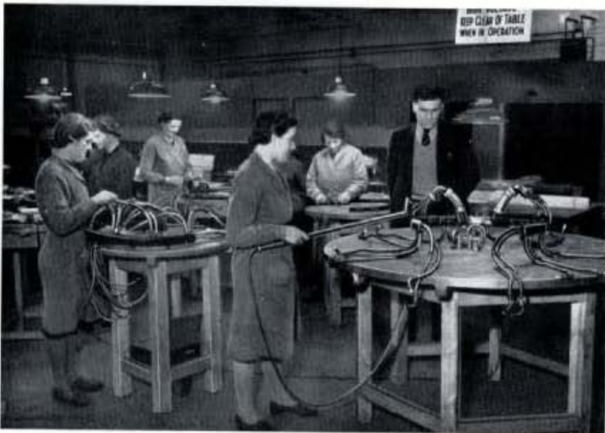
Fig. 264—Electrical harness assembling and testing; the woman at the right hand metal covered round table tests each cable at a voltage varying from 10,000 to 15,000 using the wander prod as indicated.
