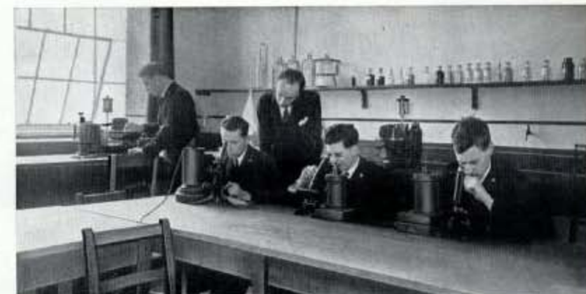
Fig. 133—A corner of the new Metallurgical Laboratory in which Air Engineer Officers are examining ferrous and non-ferrous material specimens under the microscope, after polishing and etching.
