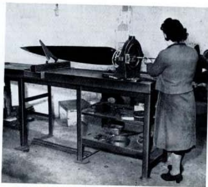
Fig. 230—The pin setting on a Rotal propeller blade being operated to provide the best geometrical position for the blade angle, which is determined by the gauge towards the tip.
