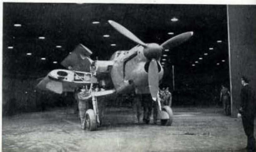
Fig. 138—A view of the Merlin on test in the Test House, complete with oil and coolant radiators. The test run is arranged to simulate all climate and altitude conditions likely to be encountered.
