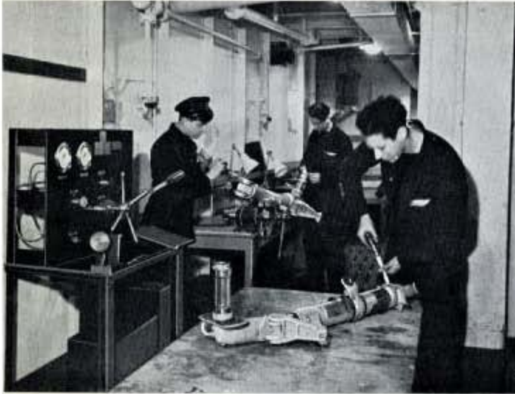
Fig. 355—The Hydraulic and Oleo Leg Repair Shop is situated on the hangar deck and here we show mechanics at work on oleo components; a Lockheed static hydraulic test rig will be seen on the left.
