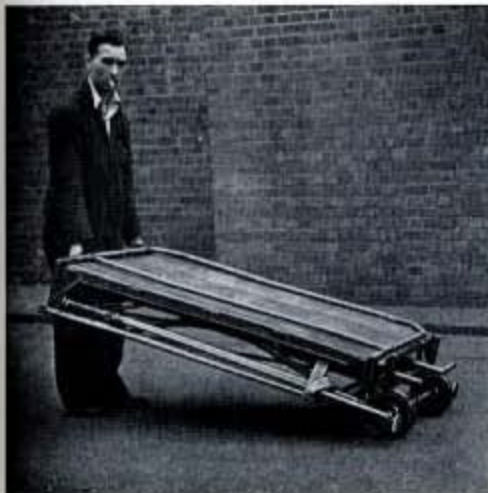
Fig. 209—A folding platform which proves extremely useful for the maintenance of aircraft.
