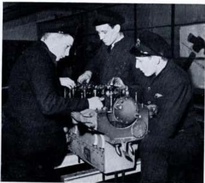
Fig. 48—G Class (3 to 3½ year period) Fitters and Turners stripping a Dorman diesel engine. When reassembled after inspecting for wear or breakage, the engine must be run by them in the next shop (See Fig. 49)
