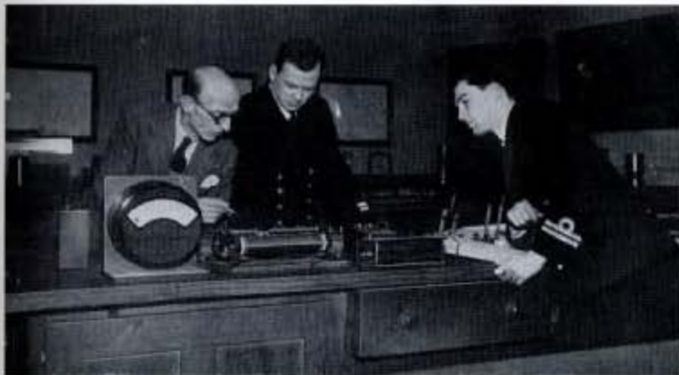
Fig. 116—Two Lieutenants (E) in their passing out terms (9th) calibrating an ammeter by means of a Crompton potentiometer under the eye of their lecturer in the Low Power Electrical Laboratory.
