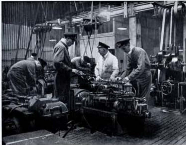
Fig. 110—As part of the general refitting instruction given to officers during their seventh and ninth terms in Workshop Practice, they have to strip down and refit various reciprocating engines.
