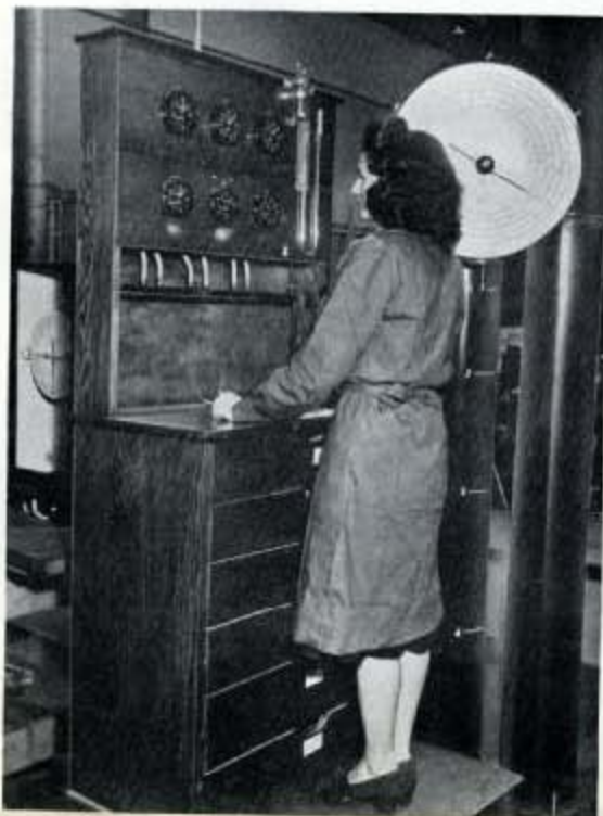
Fig. 304 (Left)—A master calibrator in use for testing air speed indicators.
