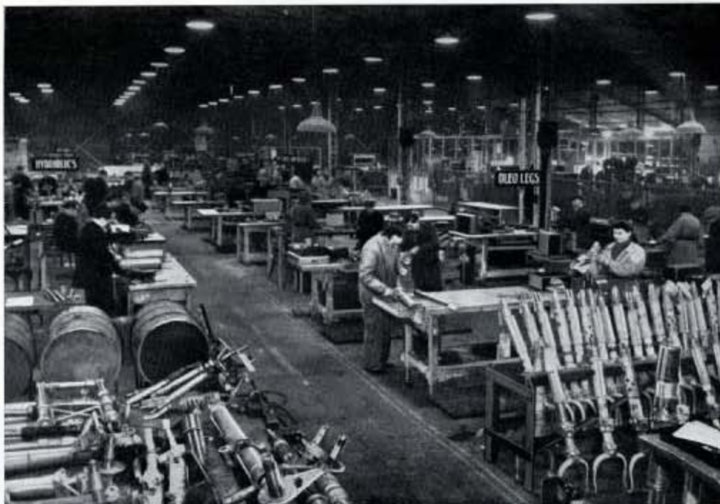
Fig. 267—A general view in the Component Repair Bay of the Mechanical Workshops; here are sections for the repair and test of oleo legs, cocks and filters, hydraulic and pneumatic equipment etc., a welding section is also included.
