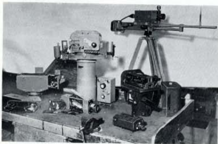
Fig. 310—Some of the types of aircraft cameras which are completely overhauled and tested to a rigorous specification before releasing for further service.
