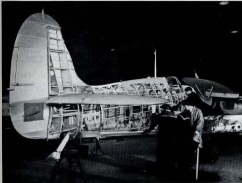
Fig. 166—Sectionalised aircraft such as this Seafire is one of the features of the instructional training at Worthy Down; on these all maintenance ratings, i.e. airframe (A), engine (E), electrical (L) and ordnance (O) are taught the operations pertaining to "between flight," "daily" and "40 hour" inspections.
