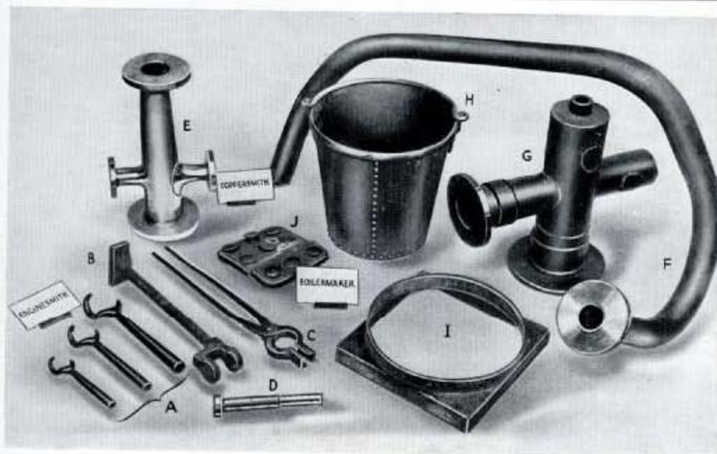
Fig. 66—Standard half yearly test jobs for Boilermakers, Enginemen and Copper-smiths. (The lettered references are given in the text below).
