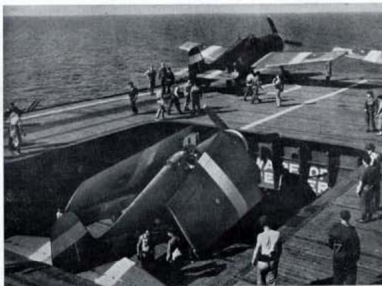
Fig. 337—A Hellcat comes up to the flight deck of an escort carrier after servicing in the hangar below.
