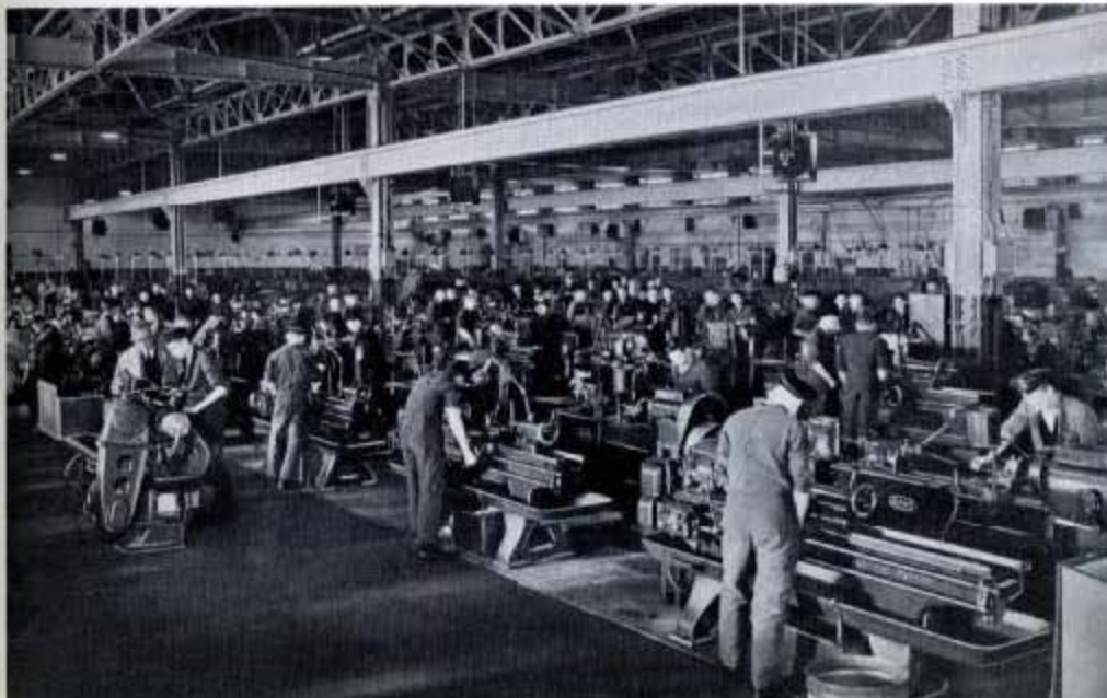
Fig. 32—Another view in the extensive Machine Shop featuring a row of Lang 13" Junior Lathes in the foreground; several Ward 1A Capstan Lathes with air chucks are installed, one of which can be seen to the left of the picture.
