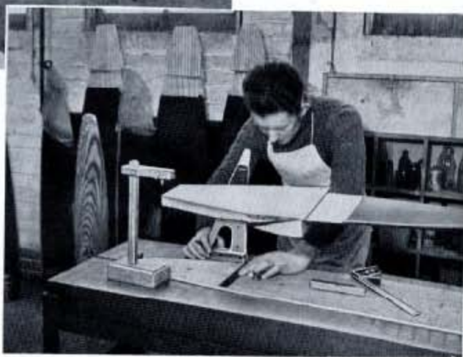
Fig. 228—Marking off a repaired wood Weybridge propeller blade for use on a Seafire; the template is secured to the table.
