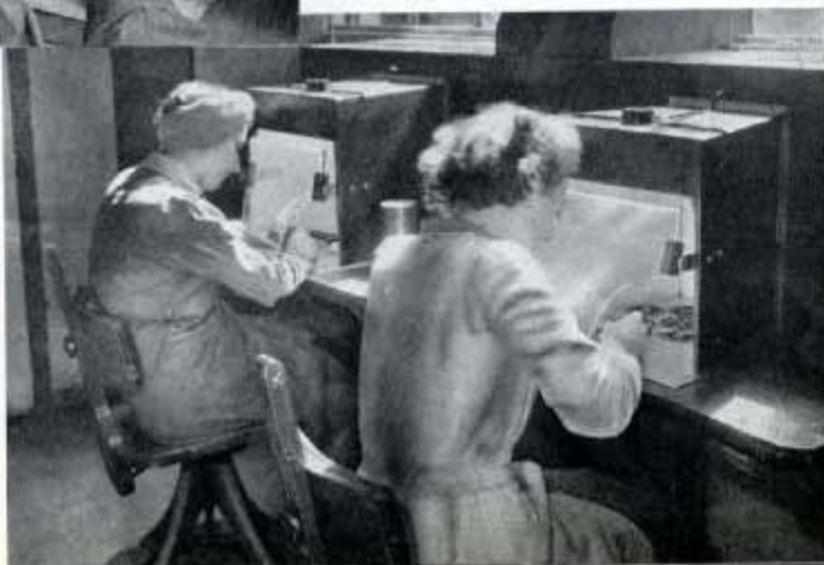
Fig. 308 (Right)—A view in the Luminising Room where the more important control instruments have their hands and dials treated with radioactive luminising paint.
