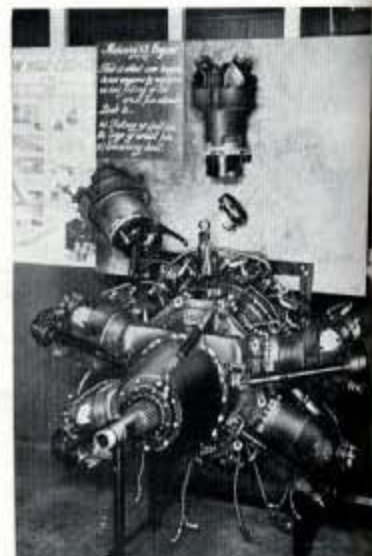
Fig. 171—The notice above this damaged Mercury engine reads—'This is what can happen to an engine by negligence in bad fitting of the wrist pin assembly. Look to (a) fitting of split pin, (b) size of wrist pin and (c) securing bolt'.
