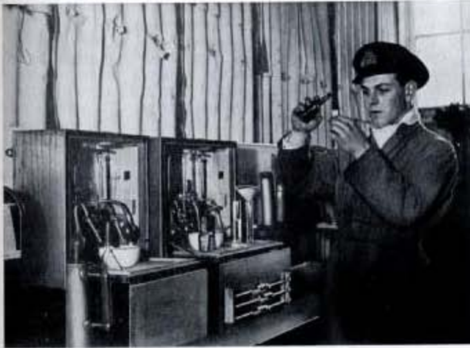
Fig. 115—The testing of boiler and feed water is done in the Engine Test Shop. By means of this equipment it is possible to determine the quantitative alkalinity and salinity of the water used.
