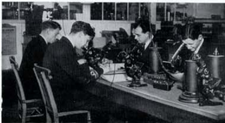
Fig. 120—Eighth term officers in the Metallurgical Laboratory making microscopic examinations of the crystalline structure of aircraft exhaust valve steels which should be particularly resistant to corrosion.
