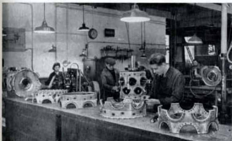
Fig. 253—Our story of the work of the E.R.S. now brings us to the assembly of crankcases and crankshafts as illustrated.
