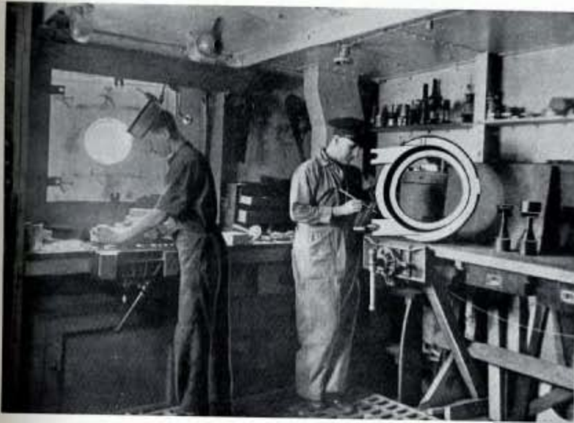
Fig. 156—Putting the finishing touches to a pattern or a new door for a washing machine in the Repair Ship's laundry.
