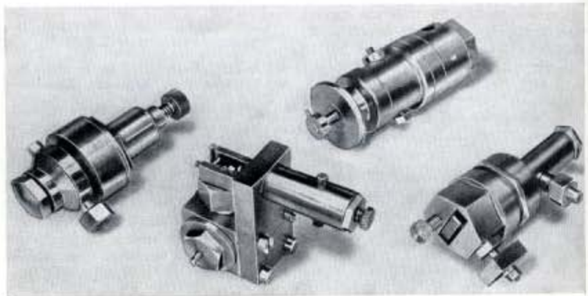
Fig. 64—A group of the four Admiralty passing out test jobs for Electrical Artificers, taken particularly to show the trip governor servo valve (second from left) seen exploded in Fig. 63.
