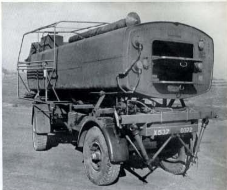
Fig. 329—This Bakery Trailer, with a capacity for 144 2 lb. loaves in a baking cycle of 70 minutes, is but one of the many specialised vehicles which go to make up a M.O.N.A.B. unit.
