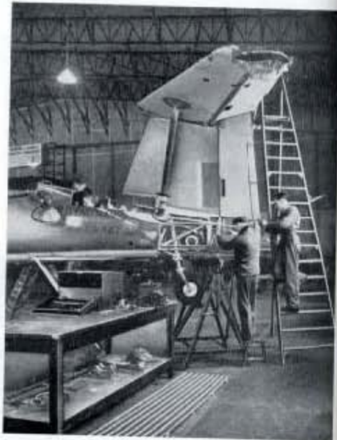
Fig. 245—Here, a Barracuda undergoing major repairs is in process of being stripped in Assembly I hangar.
