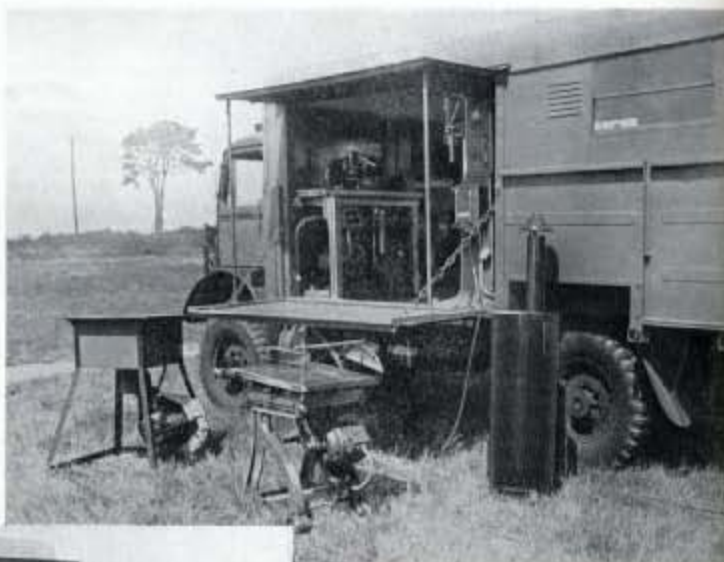
Fig. 320—The General Purpose Workshop taken from the exterior; the equipment standing outside comprises a brazing hearth, portable saw bench and salt bath.
