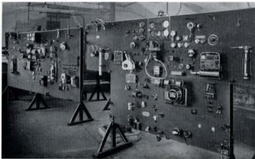
Fig. 181—Aircraft electrical circuits in full working order form part of a well-equipped section for instruction to electrical maintenance ratings. The Firefly and Barracuda panels illustrated are used for passing out petty officer air mechanics (L).
