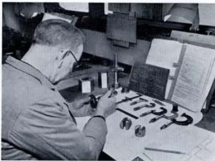
Fig. 50—Here, an instructor is marking up a circular H block, a Class G Fitters and Turners practice job, details of which are shown in the drawing Fig. 51. The system of marking is described in the text.
