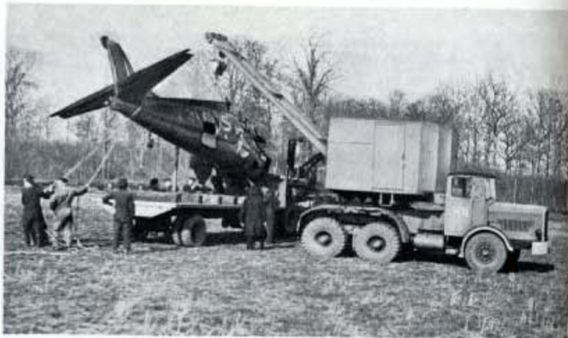
Fig. 284—A Neals 3 ton crane is used to load the fuselage on to the Cat truck, the main planes and engine being removed on a Bedford prime mover lorry (sometimes referred to as a low loader articulator).
