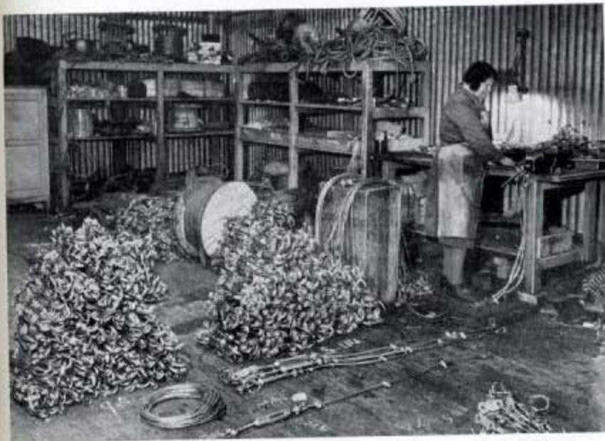
Fig. 293.—Completing sets of main securing cables prior to their final test pull of 1,200 lbs. after which they are bundled for despatch.
