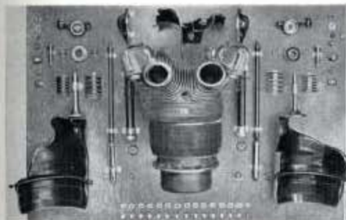
Fig. 173—The cylinder and rocker gear assembly details which commences the line of Double Wasp engine exploded sections seen in Fig. 174.
