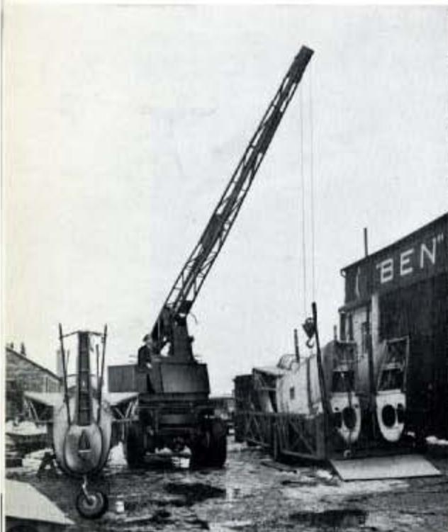
Fig. 289—An articulator arrives at the Aircraft Component Recovery Depot, Alloa with a Barracuda which is beyond economical repair, and the crane commences to unload.
