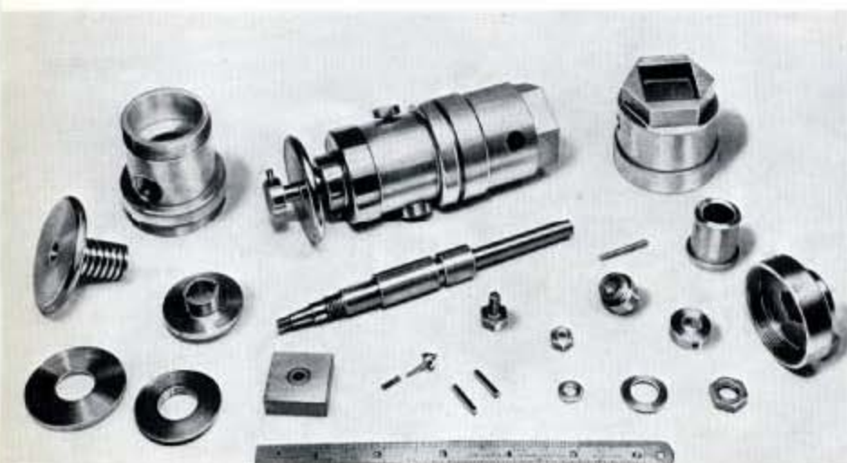
Fig. 58—This dashpot mechanism is one of the four Admiralty passing out test jobs for Electrical Artificers. For all these jobs chasers are permitted, but only a lathe or drilling machine may be used although shaping and slotting can be done in the lathe.
