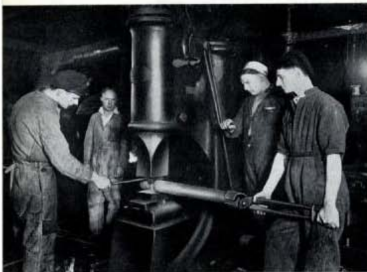
Fig. 154—Enginesmiths on board a Repair Ship using a power hammer to reduce the diameter of a steel shaft.
