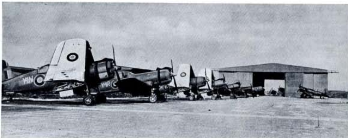
Fig. 205—Corsairs in the Reserve Pool of No. 1 M. U. undergoing daily inspection ready for re-allocation to Flights. These aircraft came in from Flights with some unserviceabilities which have been rectified and the D.I.s. are being carried out in the Pool to avoid this work immediately on returning to the Flights.
