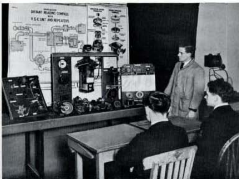
Fig. 184—Here we see instruction being given to electrical maintenance ratings on the Barracuda D.R. (distant reading) Gyro-Magnetic Compass, together with the series of repeater compasses for pilot and observer.
