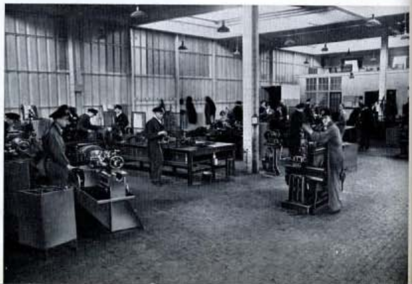
Fig. 109 (Right)—Engineer Officers in the new Fitting and Machine Shop at Manadon. Here they acquire a thorough knowledge of elementary fitting work and the ability to use all the hand tools and workshop machines usually fitted on board H.M. ships.
