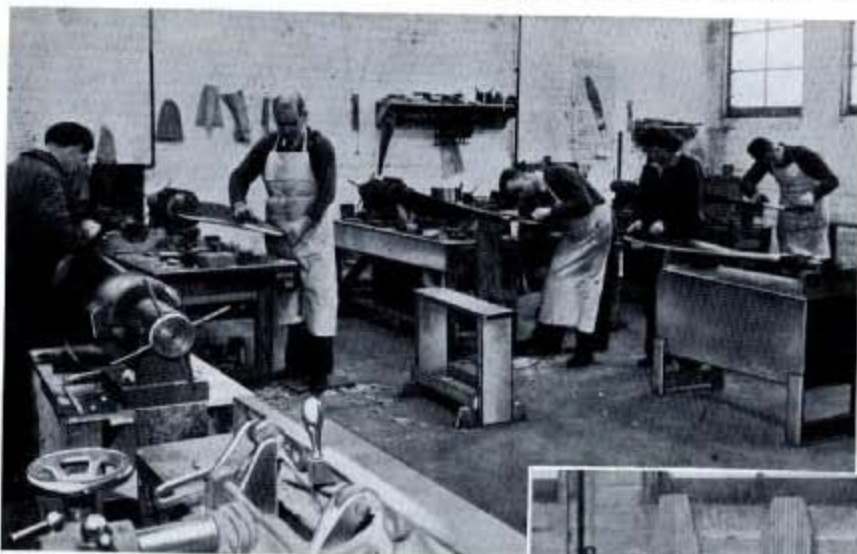
Fig. 227—General repairs in progress to wood propeller blades for Seafire and Firefly aircraft.
