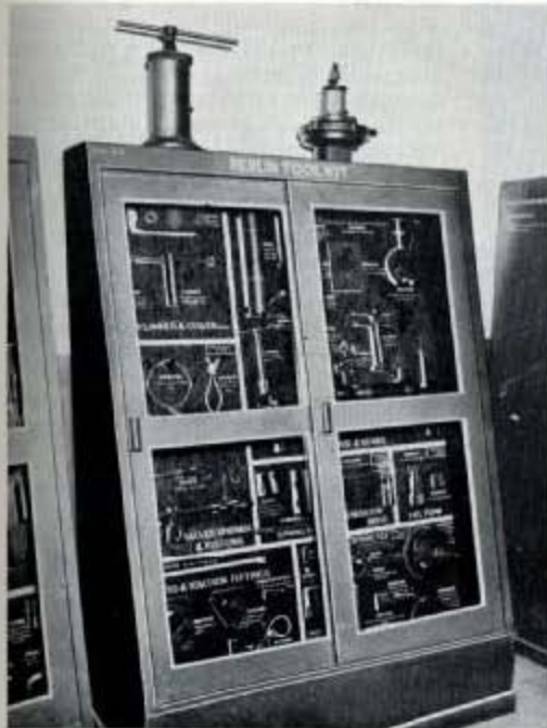
Fig. 177—This Merlin engine tool kit, one of three such cases covering the entire range, is used by officers and ratings on the Merlin engine course. Kits for other types are similarly displayed in the Instruction School.
