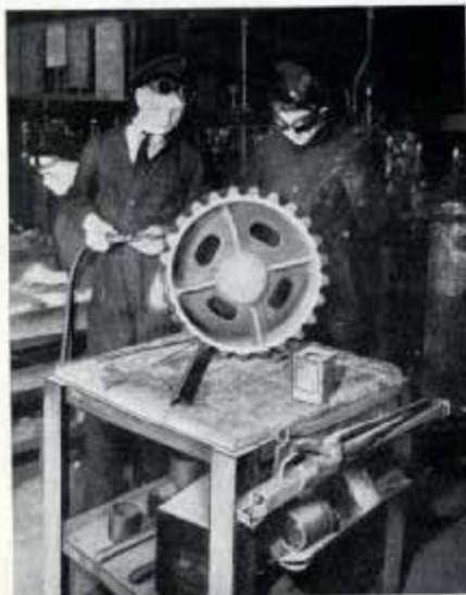
Fig. 69—Boilermaker apprentices reinforcing the worn bore of a worm wheel for the steering gear of a destroyer by oxy-acetylene welding.
