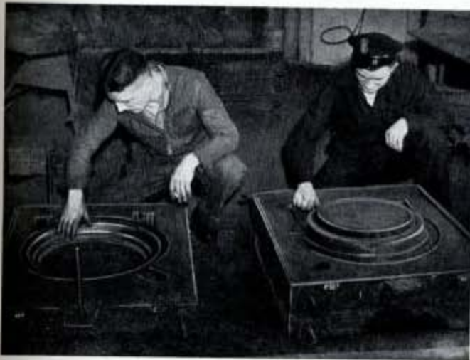
Fig. 157—Here we see the finished mould for the new washing machine door.
