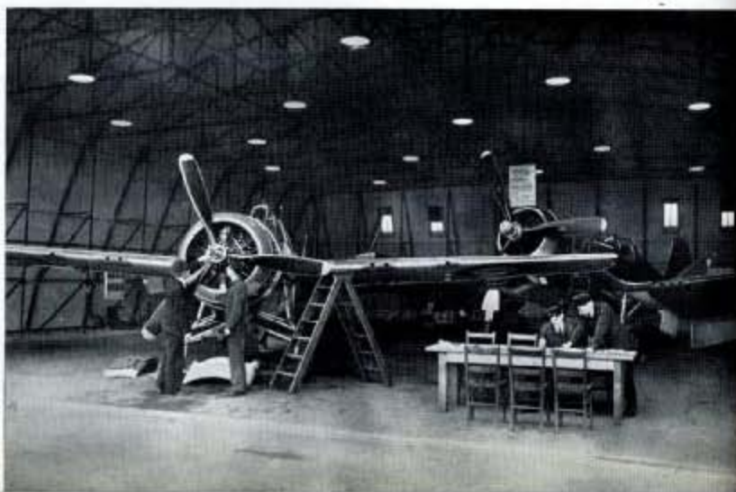
Fig. 201 (Right)—A view in the Q.S. School where ratings direct from training schools 'qualify to sign' Aircraft Servicing Form A 700 on which is recorded every inspection and repair carried out on an aircraft
