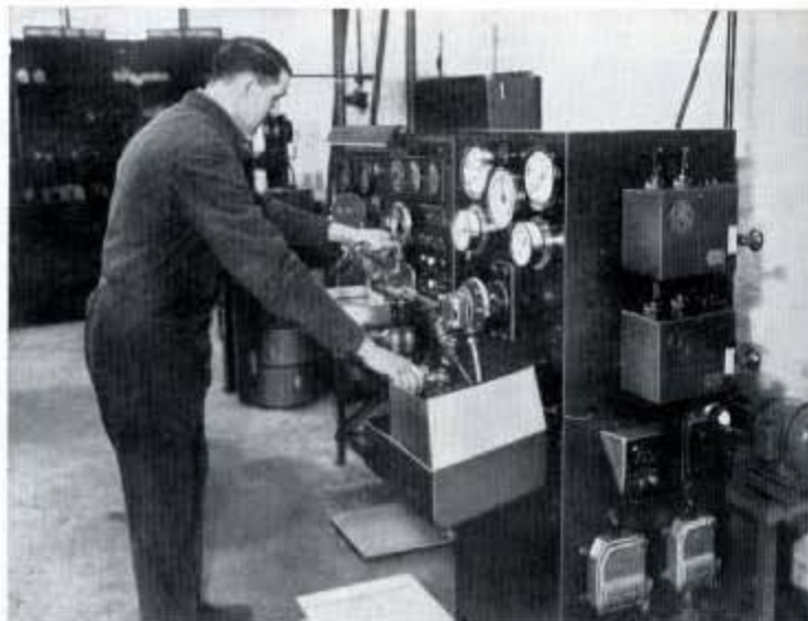
Fig. 236—Testing the constant speed governor unit for the Hamilton Hydromatic propeller. This unit controls the pitch of the blades, and through the blade pitch the revolutions of the engine.
