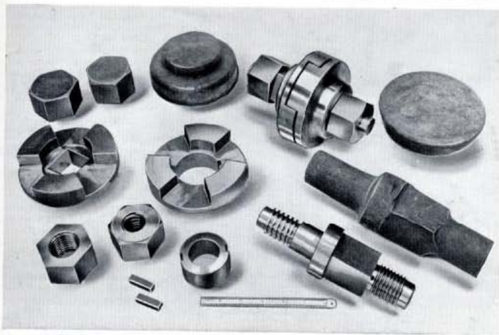
Fig. 54—The claw coupling, which is the second Fitters and Turners Admiralty passing out test job we illustrate: all these jobs are shown in their rough, machined, and assembled states, the forgings in each instance being supplied.
