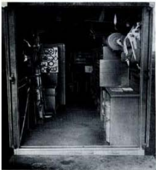
Fig. 221—This is the stores lorry of the S.S.U. which carries general aircraft and engine spares, the main control surfaces being stored in the roof.
