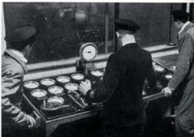
Fig. 137—A view in the control room of the new Aero Engine Test Shop. The engine on test (just seen through the plate glass) is a Merlin 30 of 1,375 rated horse power for the Barracuda I.
