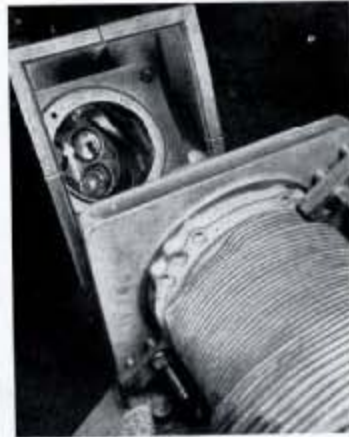
Fig. 250—On the Bristol valve seat grinders, the operator watches the grinding process on a Mercury cylinder in the mirror as indicated above.
