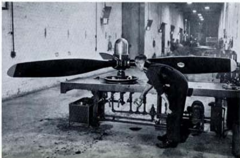
Fig. 233—To ensure correct balance, the concentricity of the Hamilton Hydromatic propeller hub must be within a maximum error of .004".
