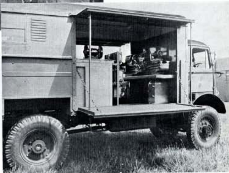
Fig. 316—This view, taken from the right hand side of the Aircraft Machine Shop, shows how the side doors let down offering extra work benches if required, as well as cooler working conditions in hot climates.
