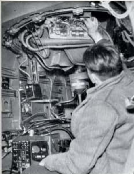
Fig. 260—Looking through the rear fuselage door into the bomb aimer's compartment of an Avenger we see an E.A.S. mechanic adjusting the elevation, train and return to neutral relays for the gun turret.
