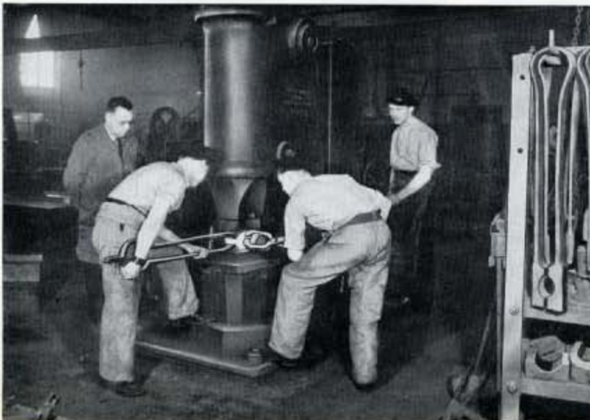
Fig. 77 (Left)—Enginesmiths (H Class) on a 5 cwt. power hammer, in the first stages of forging a connecting rod from 3½" square steel. This is one of their Admiralty passing out test jobs and is depicted at L in Fig. 78. An apprentice in C Class controls the hammer.
