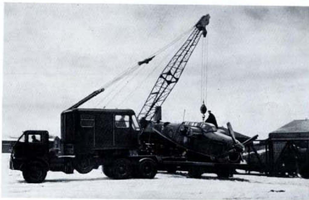
Fig. 223—A crashed Barracuda, after flak damage and subsequent forced landing, arrives at the Donibristle Repair Yard and is removed from the articulator by means of a mobile crane.
