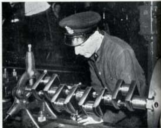
Fig. 146—Setting up a motor boat engine crankshaft in a Lang lathe prior to machining; note the stiffening bolts between the crank webs.
