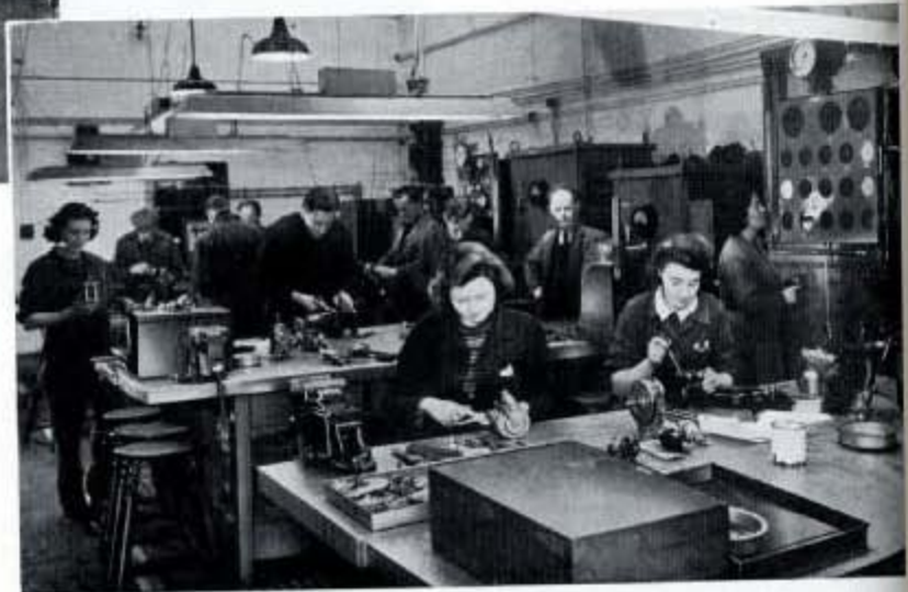
Fig. 251—Components such as oil, fuel and vacuum pumps, air compressors, magneto and generator drives are repaired and tested in this Engine Accessory Repair Section, known as the E.A.R.S.
