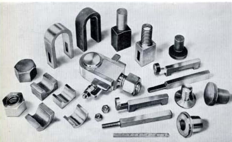
Fig. 56—This locomotive end is the last of the Admiralty passing out test jobs for Fitters and Turners: for all examples machining is done and certain excess metal removed on the lathe and shaper only, other parts have to be hand worked.
